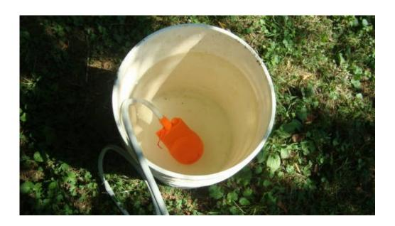
Above: The pump is inserted into a five gallon bucket filled with water. At nearly a gallon per minute run time, two five gallon buckets will provide a steady ten minute shower with good water pressure. Many different water sources will do and is left up to the user's innovation. (Not to be used in silt water or dirt filled river water)
